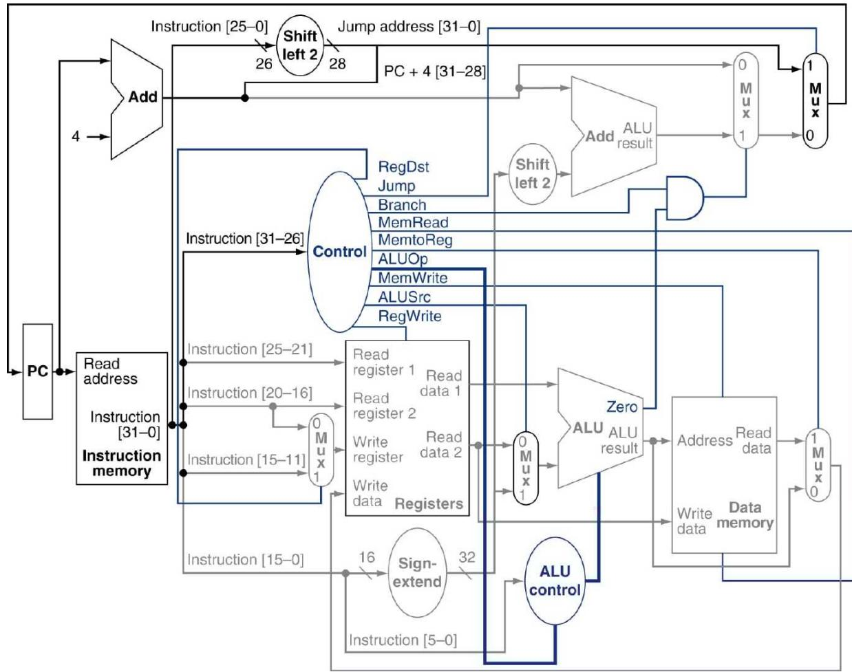
The model divides the machine into two main units: control and data paths. Each unit consists of various functional blocks, such as a 32-bit ALU, register file, sign extension logic, and five multiplexers to select the appropriate operand.
